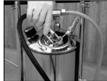
Cap is released inwards. Make sure seal does not drop into vessel.
