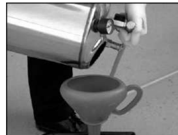
Pour cleaning agent/disinfectant into original container. Tightly seal original container.
