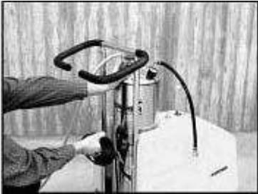
Slacken off bracket and hold pressure vessel.
